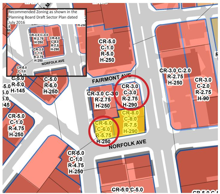
Figure 2.05: Recommended Zoning - Corrected zoning shown above for properties circled.
